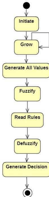
Fig 4: Activity Diagram of Constructed Model
