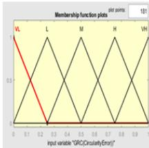
Figure 8(a) Membership function for GRC of Circularity error Cr
