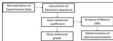
Figure 3 Procedure Adopted to Evaluate the Multiple Performance Characteristics
