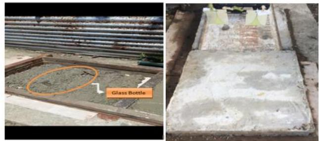
**Fig 7 With Space Void as Delaminated Portion**
