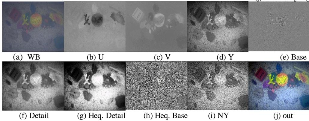
**Fig.2.** (a) white balanced image, (b)-(d) U, V, Y channels, (e), (f) base and detail layers (g), (h) histogram equalized layers (base, detail), (i) new Y channel, (j) output
