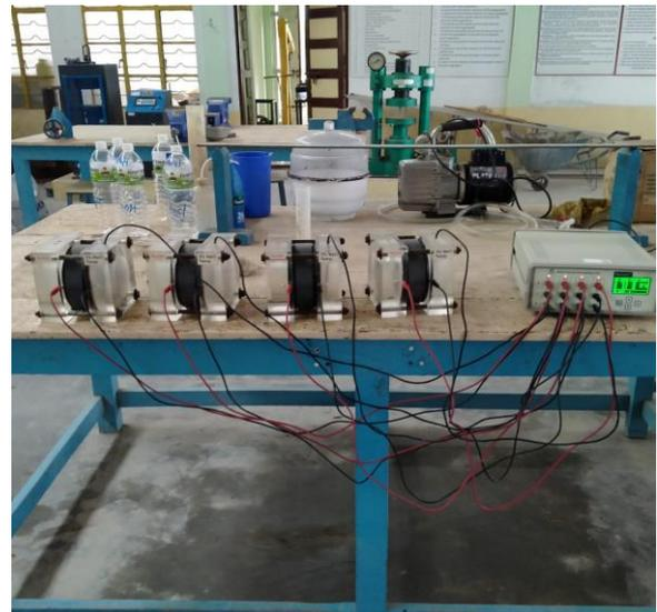
**Figure 7 Setup for a rapid chloride penetration test.**
