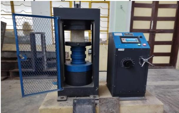
**Figure 4 Setup for compression strength test**
