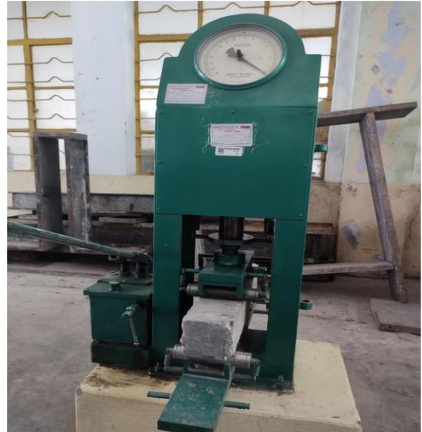
**Figure 6 Test setup of flexural strength**
