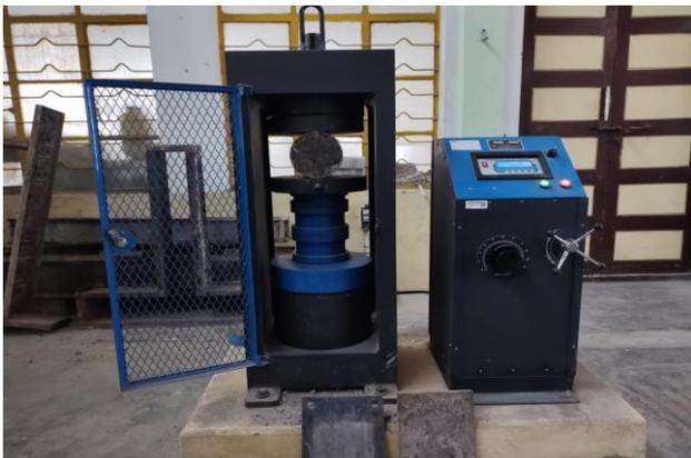
**Figure 5 Test setup of split tensile strength**
