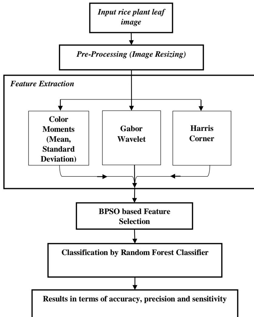
Figure 1: Block diagram for proposed rice leaf disease detection
