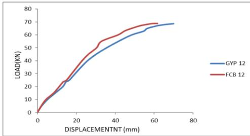
**Fig. 9.b) FCB and Gypsum board having thickness 12 mm and 12 mm**
