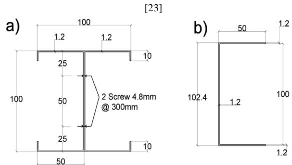
**Fig. 2. Cross-section details of a) stud and b) track**
