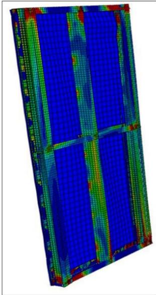
**Fig.11. Von Mises stress contour plotted on the deformed shape of FCBM16**
