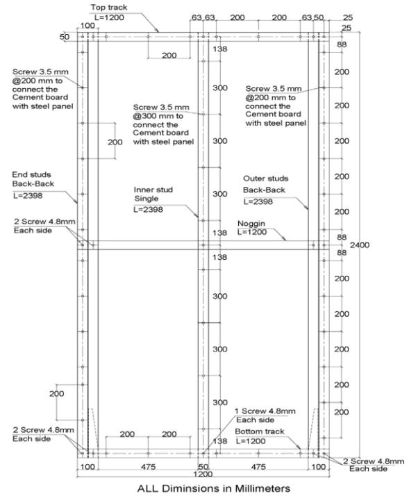
**Fig. 1. Shear wall Detailing**
