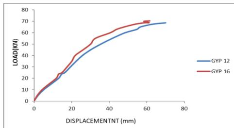
**Fig. 9.d) Gypsum Sheathing having different thicknesses**
