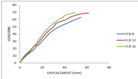
**Fig. 9.c) FCB Sheathing having different thicknesses**
