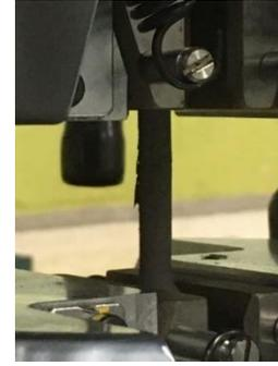
**Fig. 15: Crack in coatings within the elastic deformation of the specimen during tensile loading**
