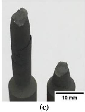
**Fig. 16: The fractured surface of; (a) uncoated steel, (b) WC-12Co coated steel, (c) WC-10Ni coated steel**
