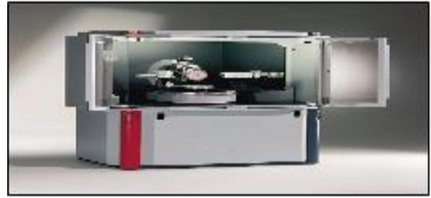
Fig 8: X-ray diffraction device
