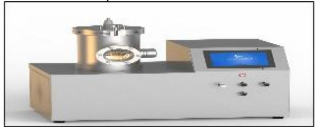
**Fig 4: Vacuum Drying Chamber**
