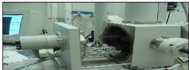
**Fig 6: Scanning electron microscope.**
