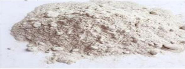
**Fig 1: Finely ground Phosphogypsum.**
