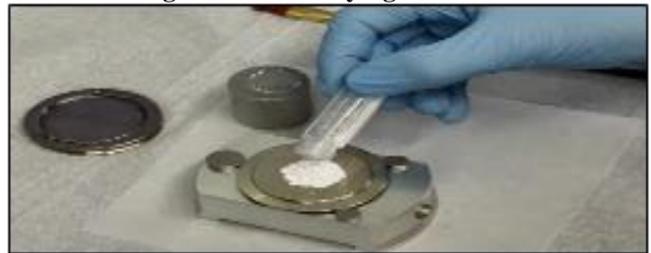
**Fig 5: SEM Sample Specimen mount preparation.**
