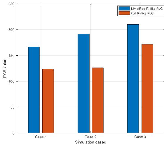
**Fig. 17: A comparison between three simulation cases only consider the PI-like FLC models**
