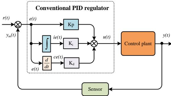
**Fig. 1: A conventional PID-based control strategy**
