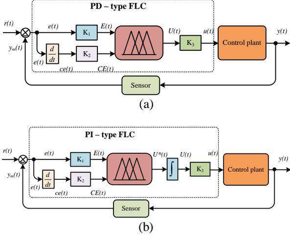
**Fig. 4: Typical architectures of control strategies applying FLCs**
