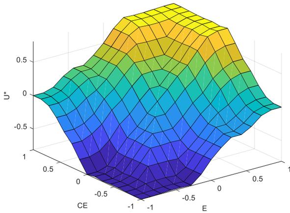
**Fig. 6: A 3-D surface of the full FLC model**
