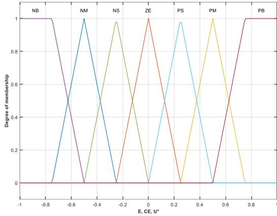
**Fig. 5: An illustration of seven membership functions for full FLC topologies**
