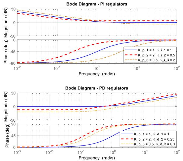
**Fig. 3: The demonstration of the dynamic responses regarding the PD and PI regulators**
