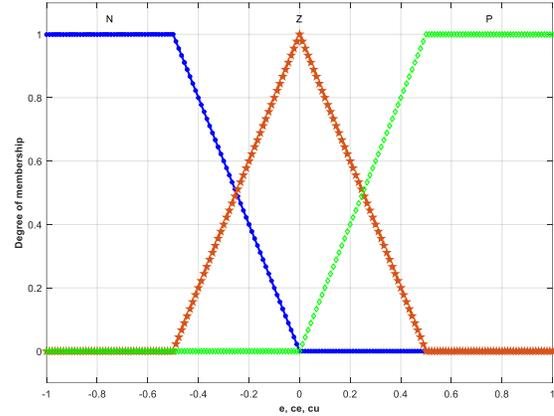
**Fig. 7: Three membership functions for two inputs and one output of the simplified FLC structure**
