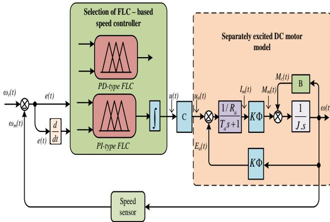
Fig. 9: A case study of applying two FLC models
