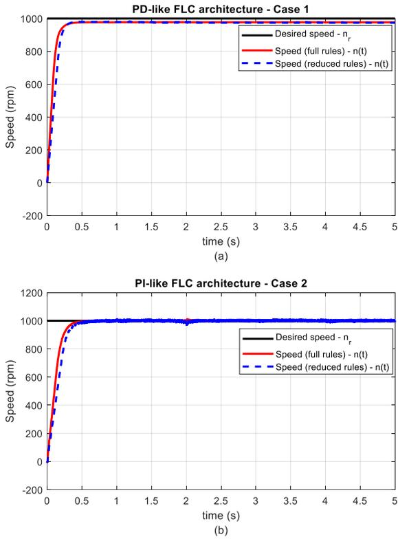
**Fig. 13: Simulation results for the second case of  $T_L$**
