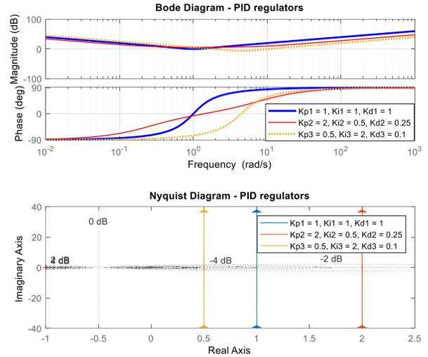
**Fig. 2: An illustration of the dynamic responses regarding the PID regulators**
