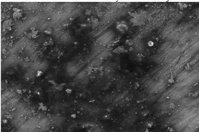
**Fig. 11.a SEM image welded joint at 450 rpm and 16 mm/min with the conical tool.**
