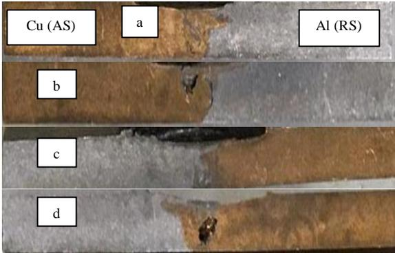
**Fig. 5 Defects in various welding process parameters**
