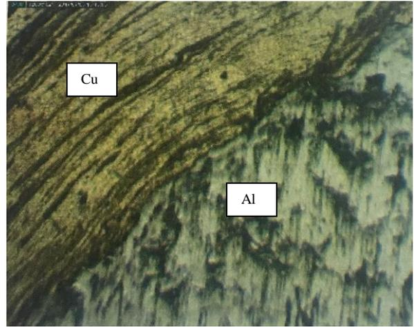
**Fig. 7 Microstructure conditions of the welded joint at 560 rpm and 16 mm/min with the conical tool.**
