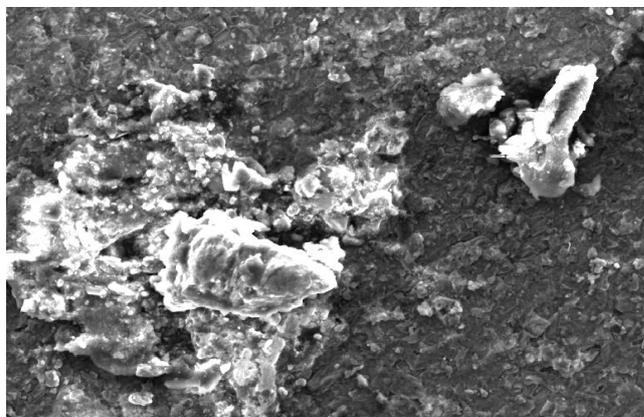
**Fig. 11.e SEM image welded joint at 450 rpm and 16 mm/min with the cylindrical tool.**
