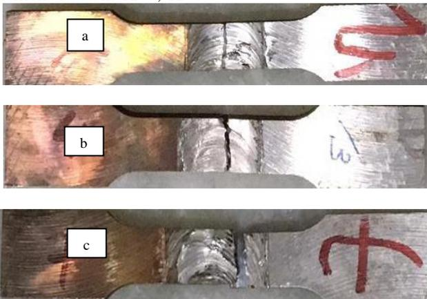
**Fig. 12 (a, b, c) Fractography at various conditions**
