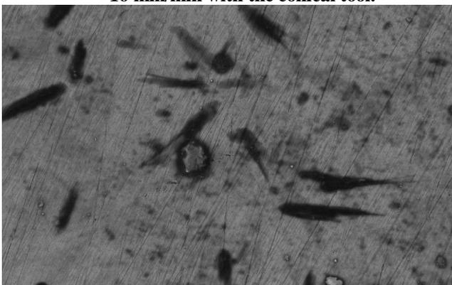
**Fig. 11.b SEM image welded joint at 560 rpm and 16 mm/min with the conical tool.**
