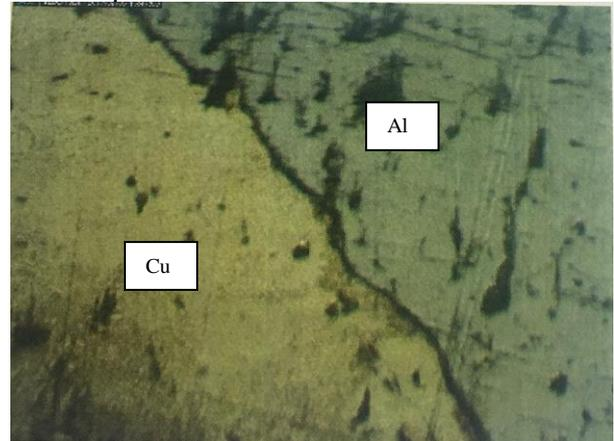
**Fig. 8 Microstructure conditions of the welded joint at 710 rpm and 16 mm/min with the conical tool.**
