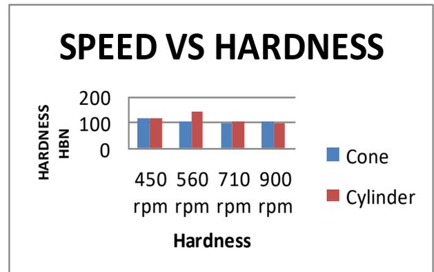
**Fig. 15 Hardness at different speeds**
