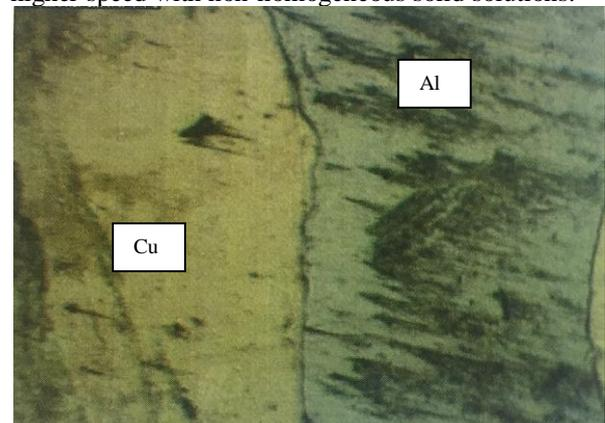
**Fig. 9 Microstructure conditions of the welded joint at 900 rpm and 16 mm/min with the conical tool.**
