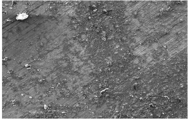
**Fig. 11.c SEM image welded joint at 710 rpm and 16 mm/min with the conical tool.**
