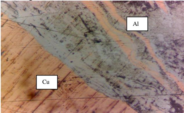
**Fig. 10 Microstructure conditions of the welded joint at 450 rpm and 16 mm/min with the cylindrical tool.**
