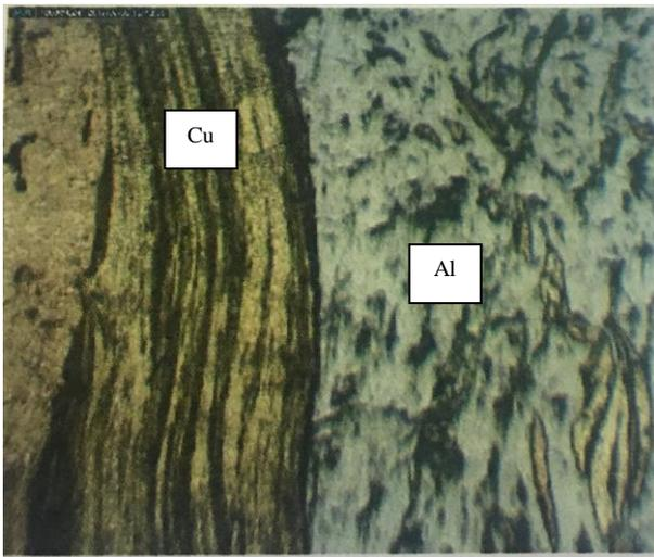
**Fig. 6 Microstructure conditions of the welded joint at 450 rpm and 16 mm/min with the conical tool.**
