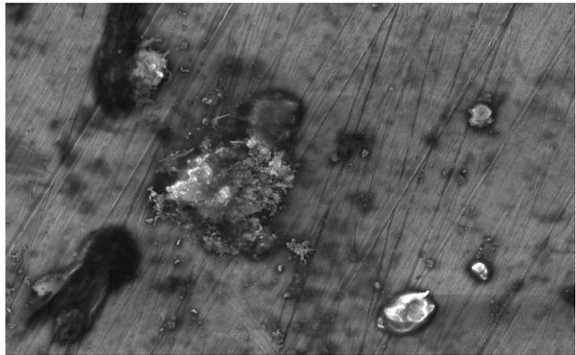
**Fig. 11.d SEM image welded joint at 900 rpm and 16 mm/min with the conical tool.**
