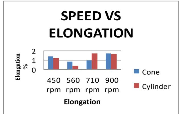
**Fig. 14 Elongation at different speeds**
