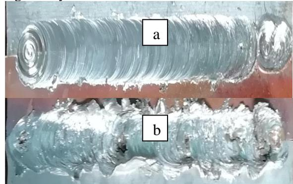
Fig. 4 Top surface of FSW welded joints using
