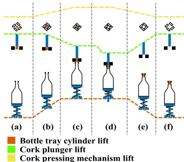
**Fig. 1: Schematic representation of the corking process.**
