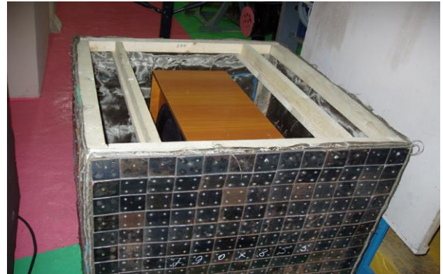
Fig. 4. General view of an experimental sound-insulating volume (a cube with sides of 1 m) with a low-frequency casing (metal plates mounted on a rubber sheet) with the top cover removed and with a sound column installed inside.
