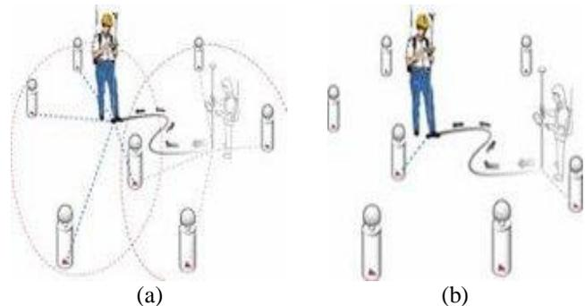
**Fig. 1 Real-time correction from permanent stations: area correction (a), Nearest correction (b).**(Images taken from the website:
