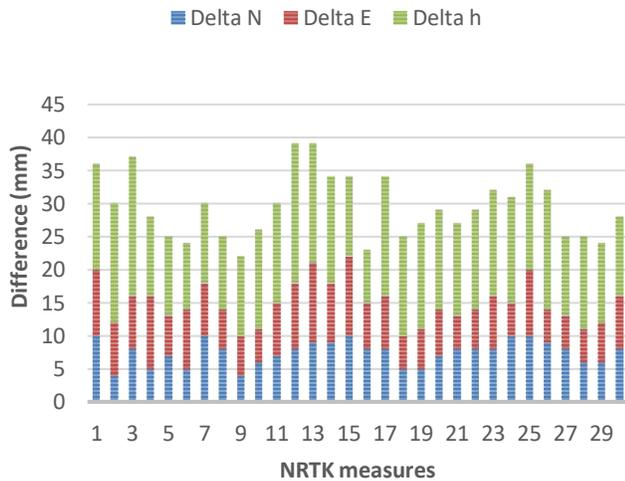
**Fig. 3. Difference of the single coordinates than a reference point.**
