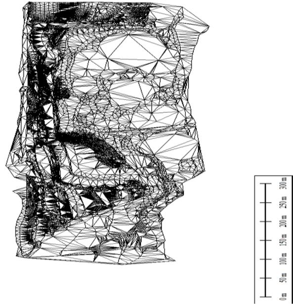
Fig. 7. TIN model of the quarry.
