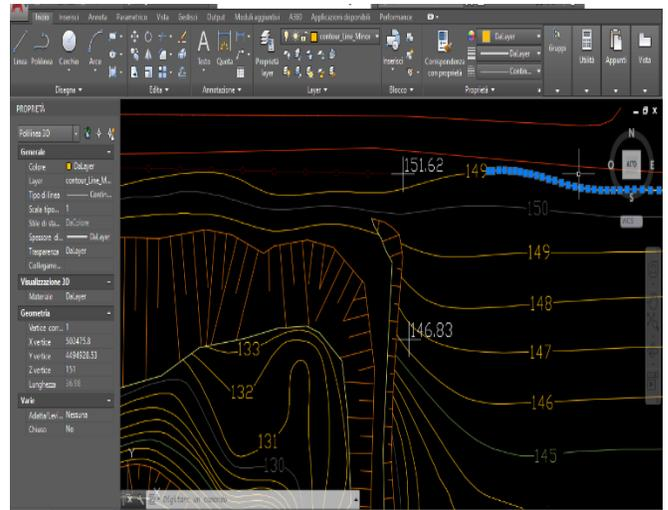
**Fig. 5. Representation in CAD environment of (part of) the quarry: 3D polyline to manage the altimetry data.**
