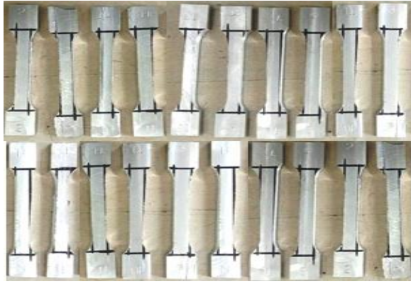
Figure 3: Dumbly shaped cut along dwell surface for UTM
