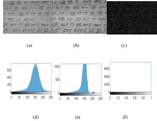
**Figure 8. Histogram analysis results (a) Original image 1 (b) Enhanced image 1 using proposed 2D EPAWABF algorithm (c) Squared error image 1 (d) Histogram of original image 1 (e) Histogram of enhanced image 1 (f) Error histogram of image 1**
