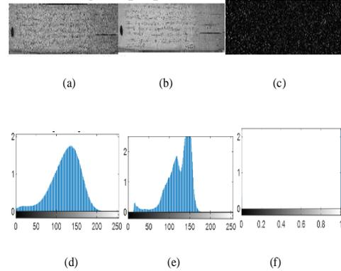
**Fig. 9. The histogram investigation results (a) Original image 2 (b) Enhanced image 2 using proposed 2D EPAWABF algorithm (c) Squared error image 2 (d) Histogram of the original image 2 (e) Histogram of the enhanced image 2 (f) Error histogram of image 2**
