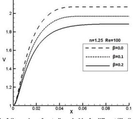
Fig. 3 Comparison of centerline velocities for different Slip Coefficient (β)
