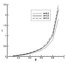
Fig. 6 Relation between Slip Length and Slip coefficients
