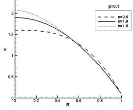
Fig. 4 Velocity profiles of slip flow through microchannel for the different flow behaviour index
