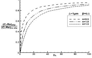
Fig. 8 Effect of hydraulic diameter (D<sub>h</sub>) on Poiseuille No. (C<sub>f</sub>.Re)
