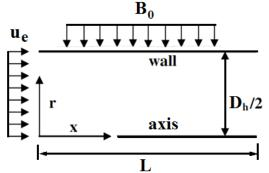
Fig. 1 Fluid domain of circular microchannel with the externally applied magnetic field (B<sub>0</sub>)
