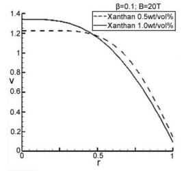
Fig. 10 Effect of concentration of Xanthan gum in Formic acid when B=20Tesla applied externally
