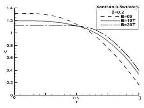
Fig. 9 the effect of the externally applied magnetic field on velocity profiles
