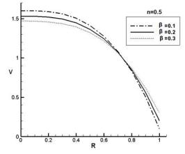
Fig. 5 Velocity profiles of slip flow through microchannel for different slip co-efficient
