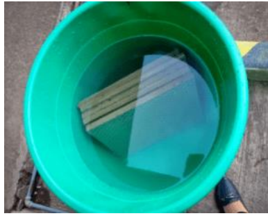
Fig. 6 The curing of tile specimens by soaking in water
