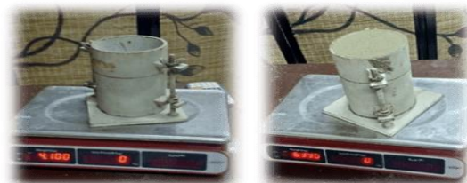
Fig. 7 (a) Weighing the empty cylinder mould and (b) weighing the mould filled with expanded perlite-based mortar for unit weight determination.
