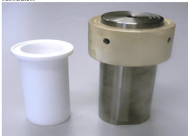
Fig. 1 Hydrothermal process autoclave
