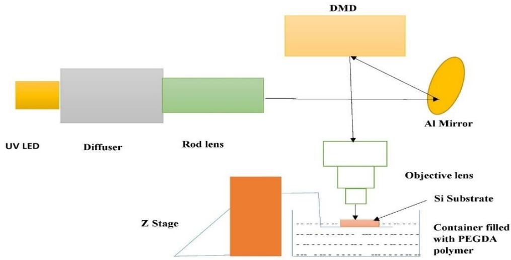
Fig. 4 Process Flow of Entire Fabrication Process
