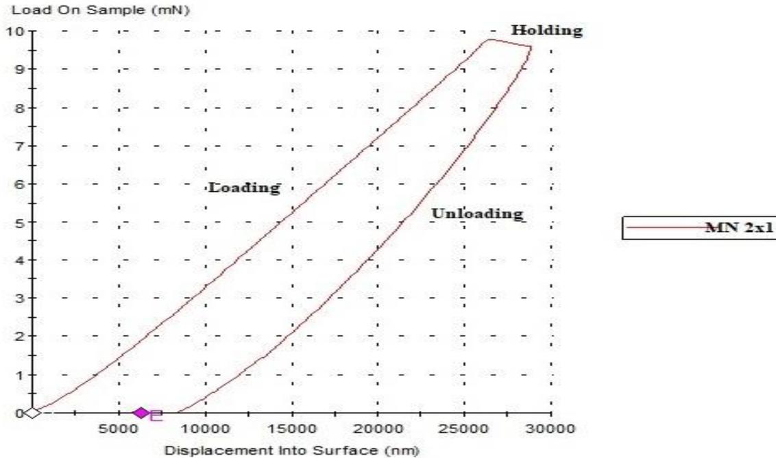
Fig. 11 Load vs. displacement curve of 2x1 microneedle at 10 mN
