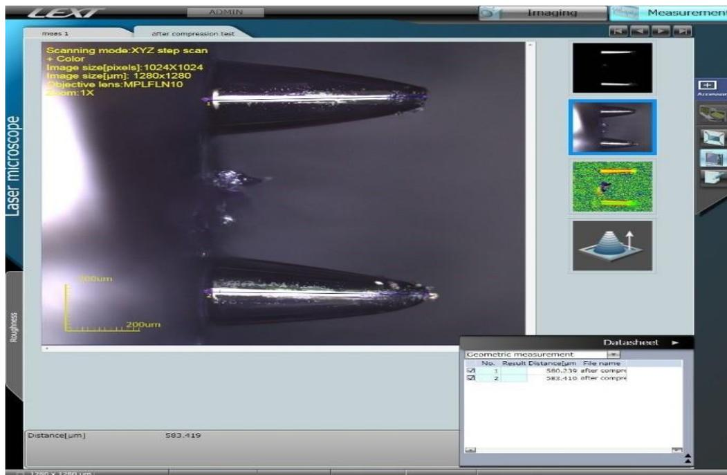
Fig. 7 Height of Cone-Shaped Microneedles
