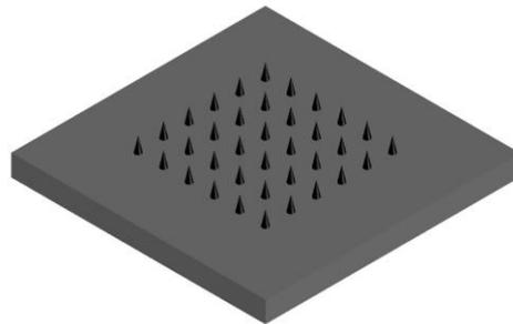
Fig. 2 Three dimensional Structure of Cone-Shaped Microneedle Array
