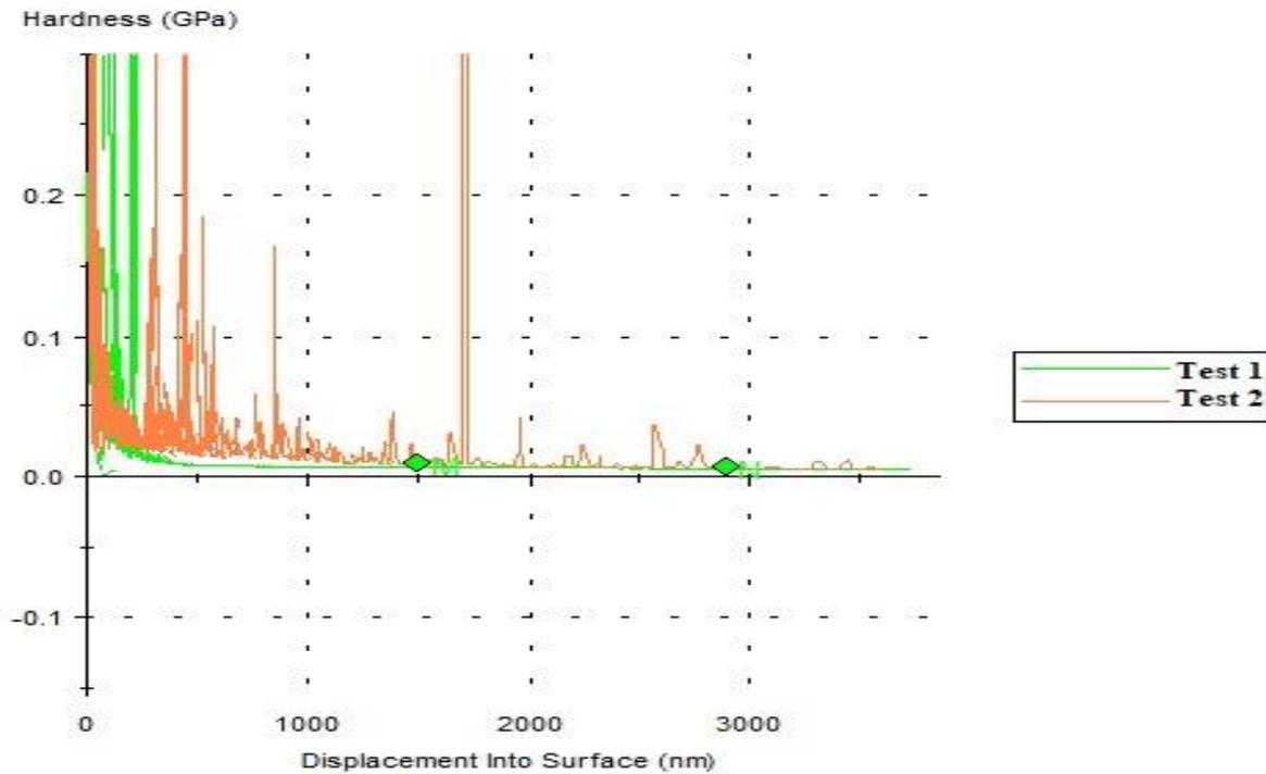
Fig. 8 Hardness of PEGDA microneedles
