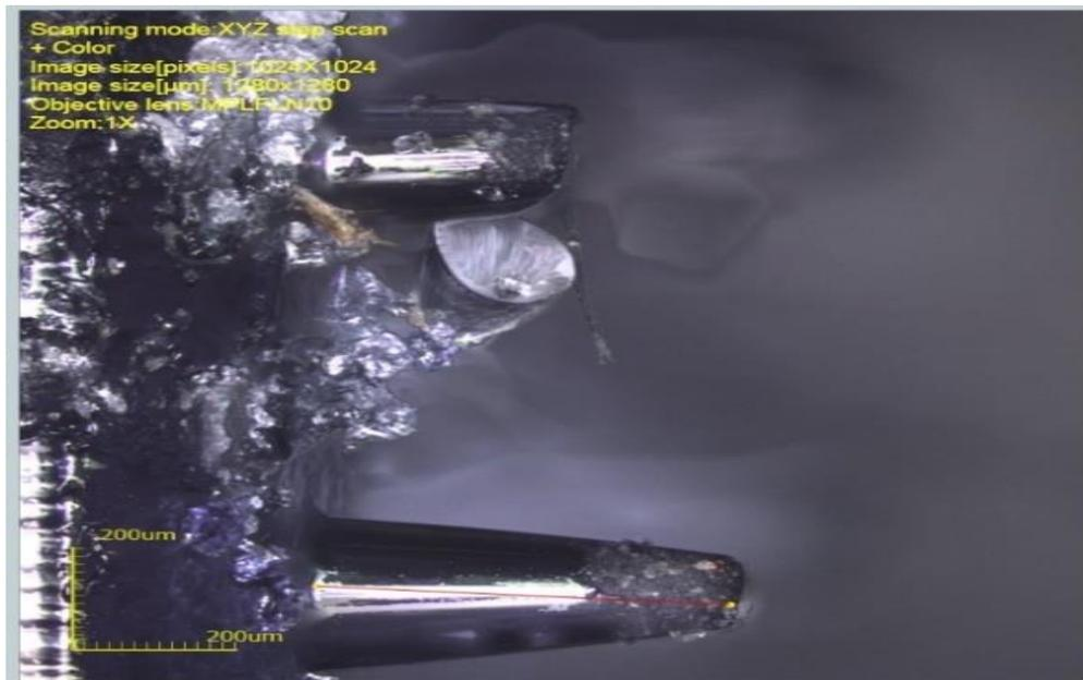
Fig. 10 Failure of the needle at 300 mN force
