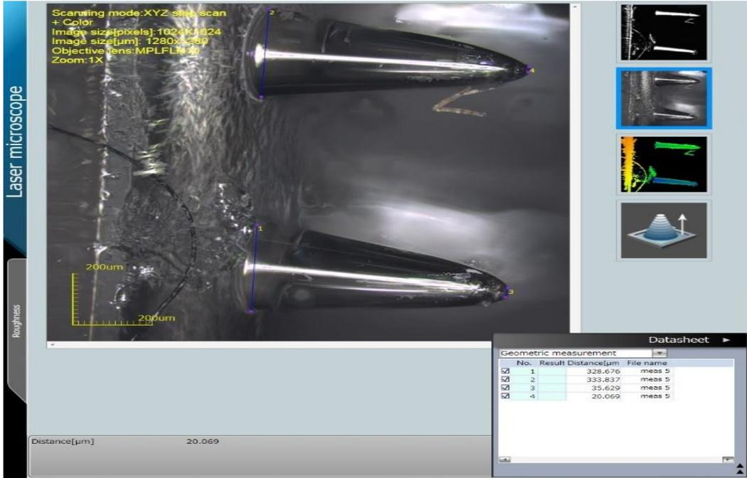
Fig. 6 Base and a Tip Diameter of Cone-Shaped Microneedles
