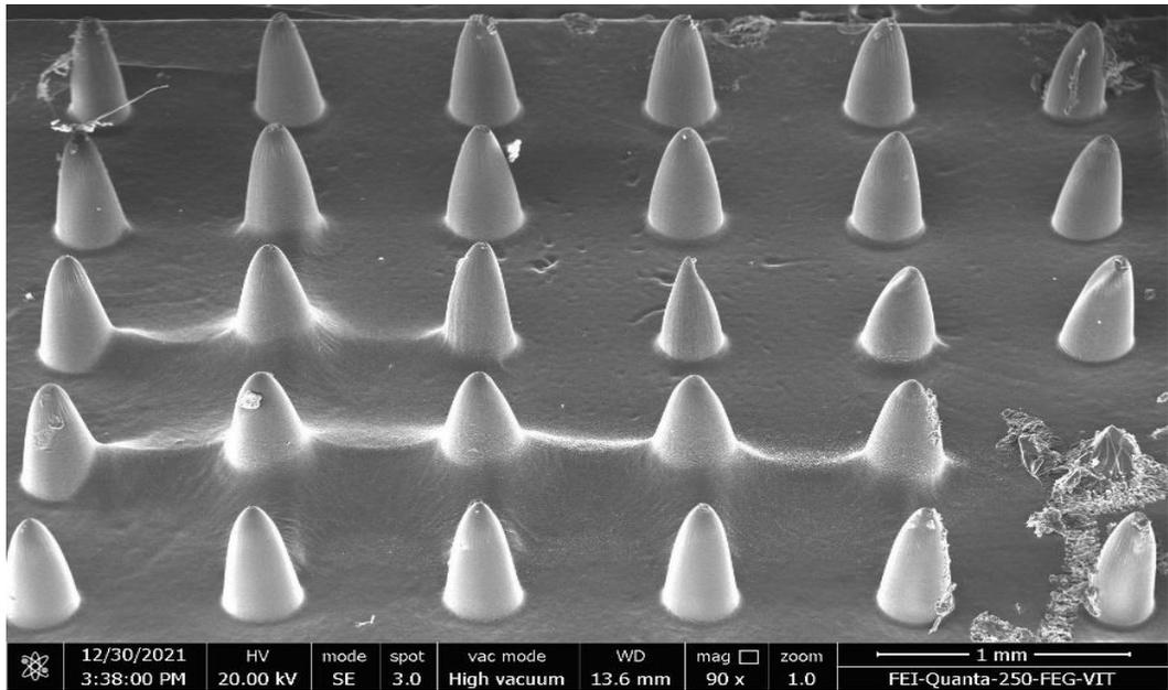
Fig. 5 SEM Images of Fabricated Cone-Shaped Microneedles Array
