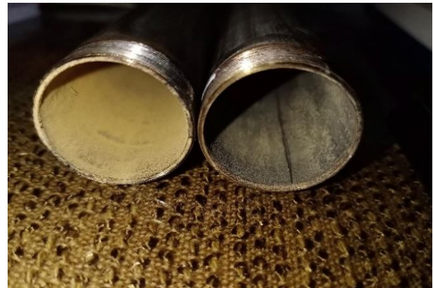
Fig. 4 Pipe without magnet having sediments, Pipe with magnet almost without sediments
