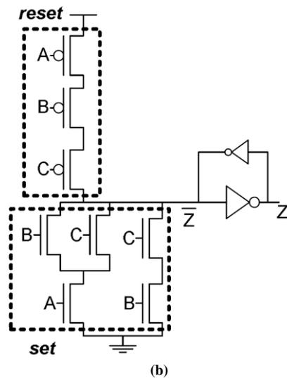
Fig. 4 TH<sub>23</sub> gate (a) Static design (b) Semi-static design
