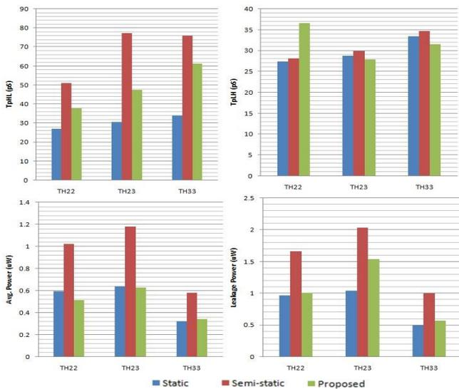
**Table 4 PDP Comparison Between Different NCL Gate Implementations With CMOS And FinFET Devices**
