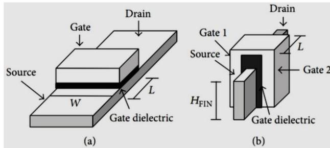
Fig. 1 Structural difference of (a) Planar MOSFET and (b) Multi-gate FinFET
