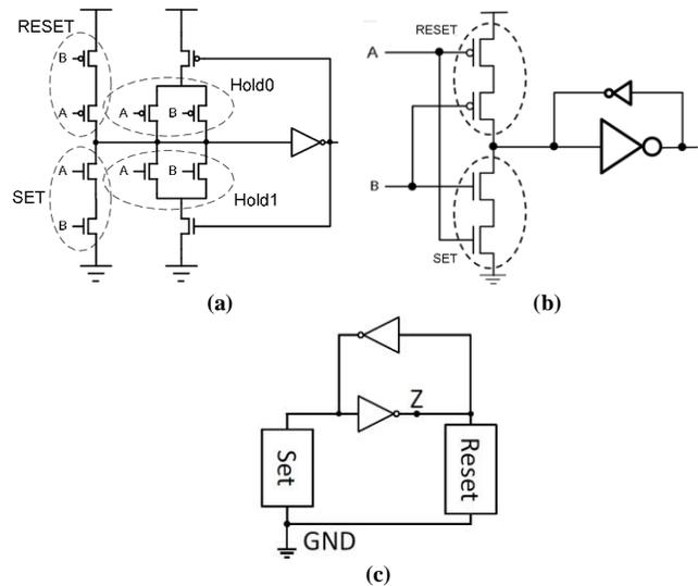
**Fig 5. TH22 gate (a) Static (b) Semi-static (c) Proposed**
