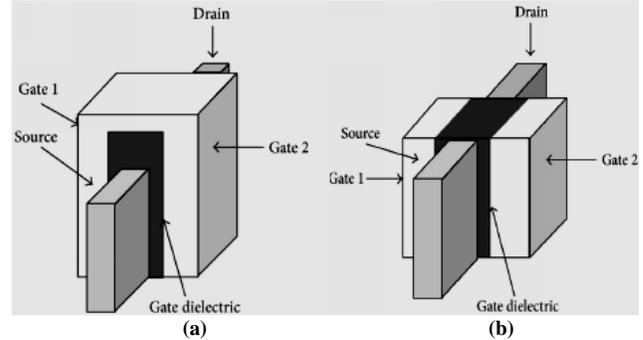
Fig. 2 FinFETs (a) Shorted Gate (SG) (b) Independent Gate (IG)
