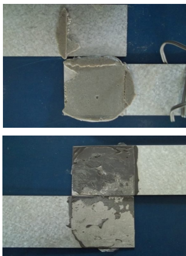
Fig. 5. Typical failure mode of adhesive joints in : a) Sikadur 31CF Normal b) JB Weld 8265 epoxy
