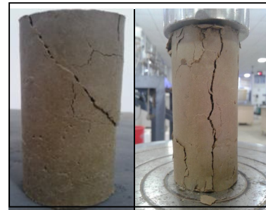
Figure 7: Failure pattern in Flyash alone & GGBS alone treated soil sample
