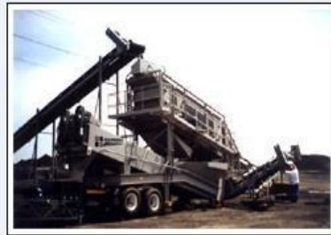
FIGURE (2): SCREENING PLANT
