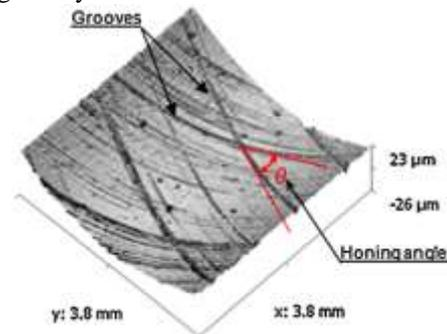
Fig 8: Plateau honed surface of thermal engine cylinder.[23]
