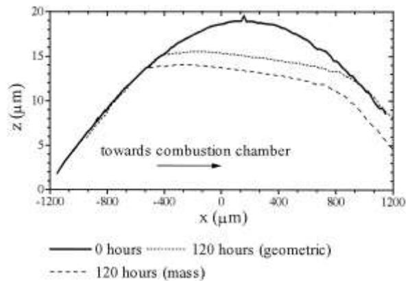
Fig 7: Measured profiles of the new and worn ring.[17]
