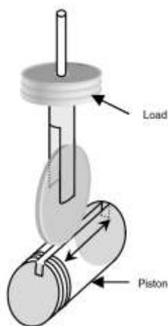
Fig 14: Loading mechanism on the piston [6]
