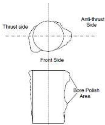
Fig 13: Exaggerated diagram of typical cylinder liner wear [6]
