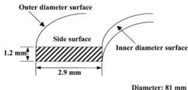
Fig 12: Typical gasoline ring dimensions [5]
