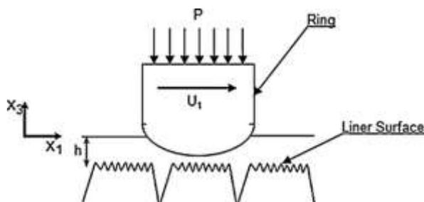
Fig 11: Piston–liner contact description[23]
