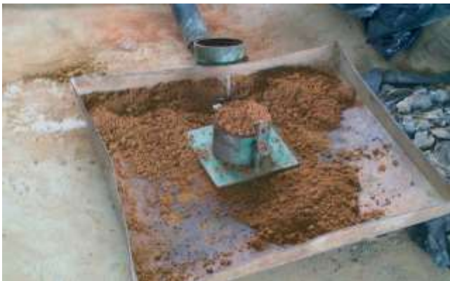
Figure 2: Proctor Compaction Mould for the compaction tests
