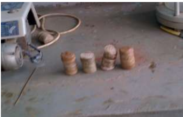
Figure 5: Photograph showing fibre reinforced test specimens after testing.
