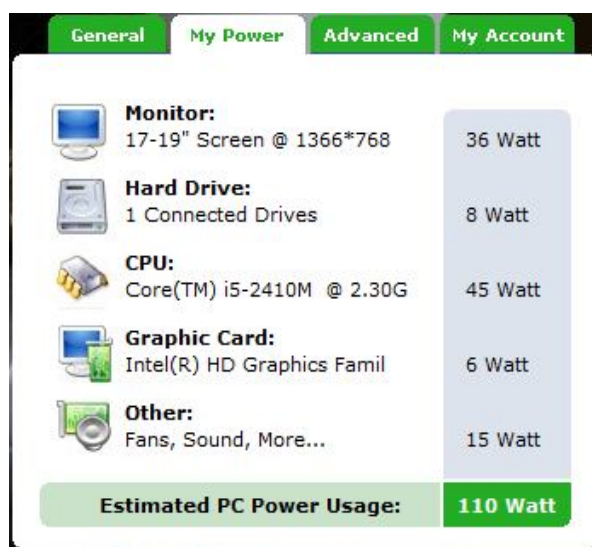
Fig 2: Power consumption of hardware devices
