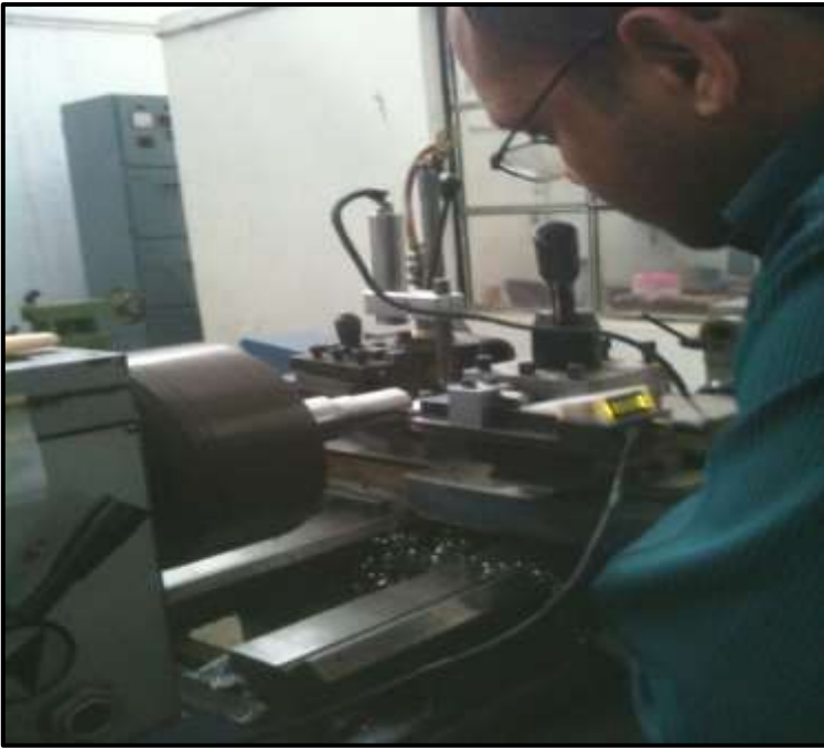
Fig.3. Experimental Setup - DRO pioneer -175 with DKM2000 dynamometer
