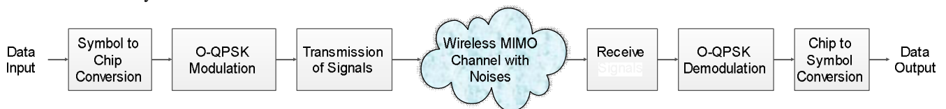
Fig. 2.1 Block diagram of the proposed IEEE 802.15.4 (Zigbee) with spatial diversity
