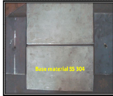
Fig.2 Specimen is tapered for weld strength.
