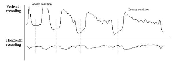
Fig. 4. EOG blink pattern for both vertical and horizontal recording originating from an alert state at the left and a very drowsy state at the right
