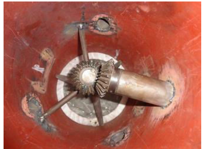
Fig. 2. The Mechanical Agitation Setup, with Blade Mounting
