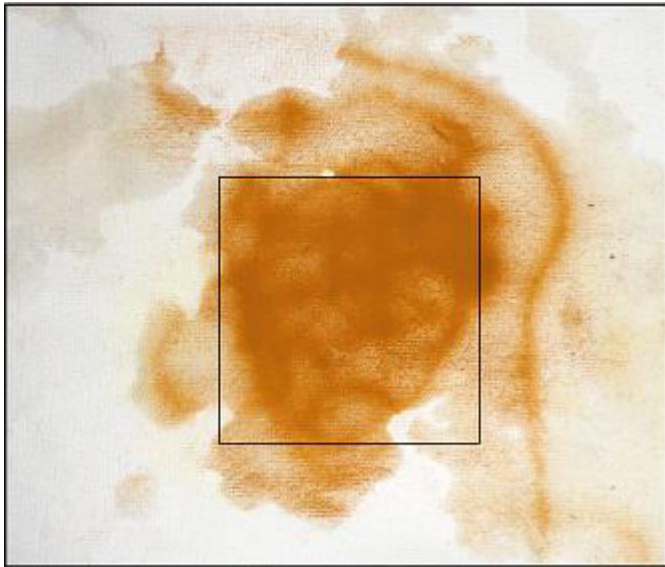
Fig. 8. Non-uniform Particle Dispersion with low-power compressor
