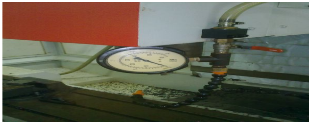
Fig. 4 Pressure Gauge attached to coolant knobe
