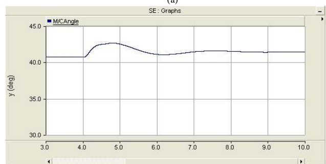
Fig.7 the shape of power angle when system is unstable (a) without HVDC Light (b) With HVDC Light
