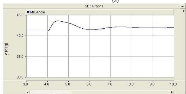
Fig.6 the shape of power angle when system is stable (a) without HVDC Light (b) with HVDC Light
