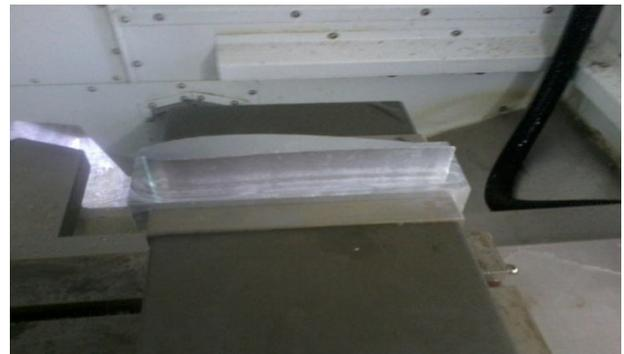
Fig. 7 Machined Turbine blade
