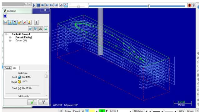
Fig. 3 Turbine blade machining: pocket (facing) operation
