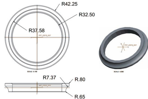
Figure 2 Model and geometry of inner race of the Bearing
