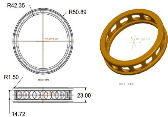
Figure 3 Model and geometry of cage of the Bearing)
