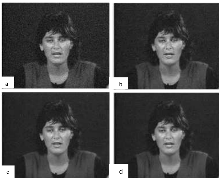
Fig. 5. Results for the 50 th frame of the denoised “Miss America” sequence. (a) Noisy image frame with \sigma = 15 ; (b) Wavelet2D filtering, PSNR=32.98dB; (c) SEQWT filter, PSNR=34.57dB; (d) Proposed method, PSNR=35.26dB.
