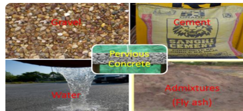
Figure 1: Materials Used in Pervious Concrete
