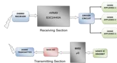
Figure1. Block Diagram of Wireless Home Automation System with Acoustic Controlling.
