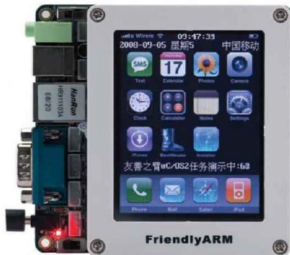
Figure 4:ARM9 GUI for controlling home appliances
