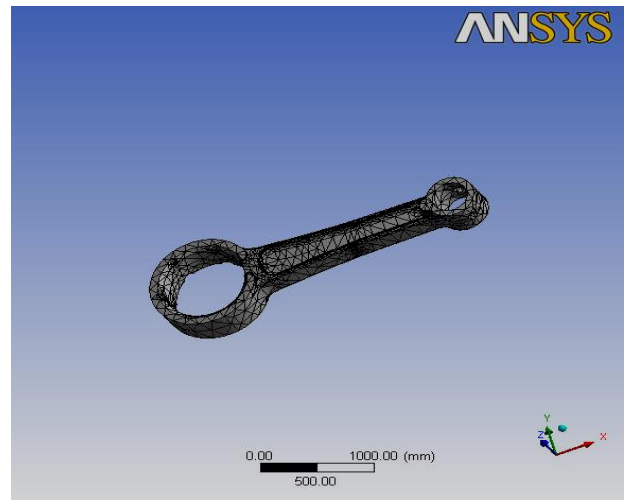
Fig 2: Mesh model of connecting rod
