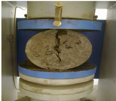
Fig. 2: Split tensile test
