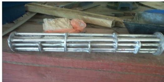
Fig 1: A picture of the tube bundle under construction with layout of about angle of 30°
