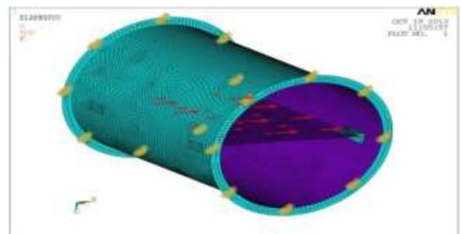
Fig 19 shows boundary conditions applied on the mounting structure for roll condition
