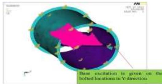
Fig 33. Shows Boundary conditions applied on the mounting structure for PSD analysis in Y-Direction
