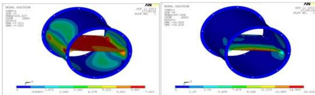
Fig 25 shows the 3<sup>rd</sup> and 4<sup>th</sup> mode shapes for modal analysis
