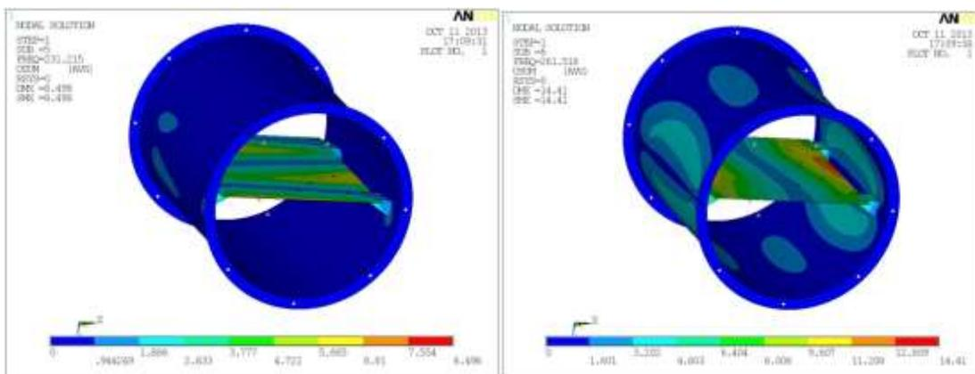
Fig 26 shows the 5<sup>th</sup> and 6<sup>th</sup> mode shapes for modal analysis
