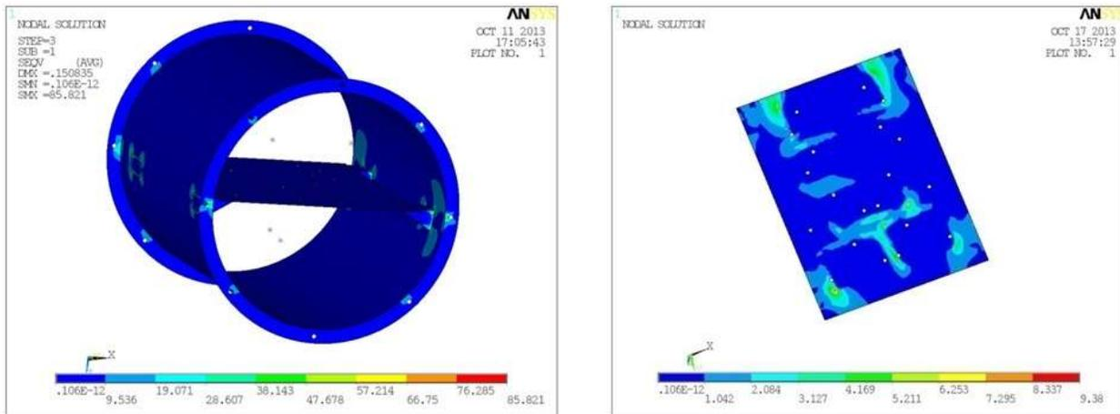
Fig 29 shows 1 sigma stress for PSD analysis in X-Direction
