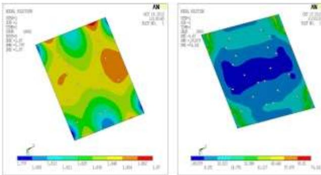
Fig 21 shows deflections & stress plot of mounting plate for roll condition
