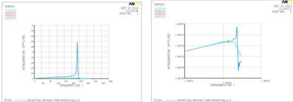
Fig 36 Shows PSD Response on plate on electronic packages in Linear and Logarithmic Scale
