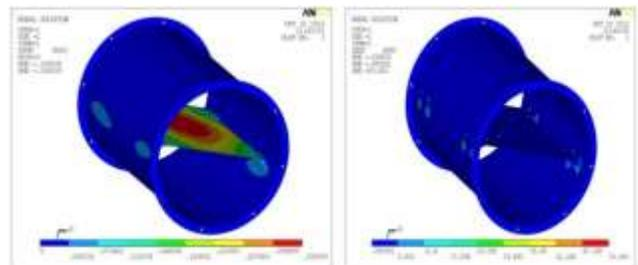
Fig 12 shows deflections & Stress plot of mounting structure for yaw condition
