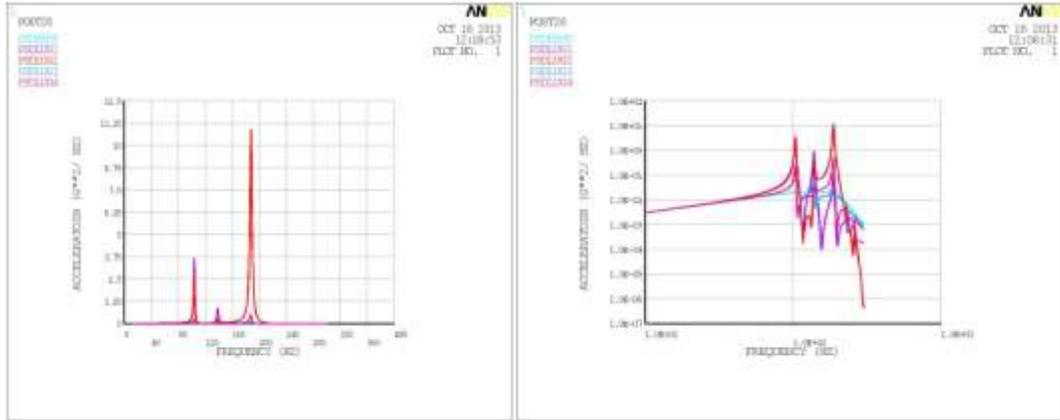
Fig 44 Shows PSD Response on lugs in Linear and Logarithmic Scale
