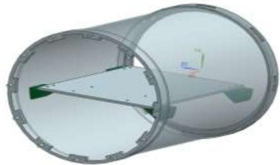
Fig 8 shows the 3d model of mounting structure assembly
