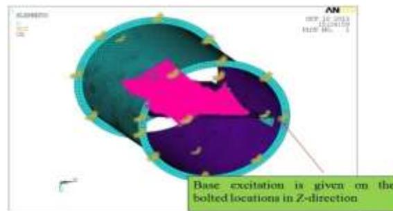
Fig 39 Shows Boundary conditions applied on the mounting structure for PSD analysis in Z-Direction
