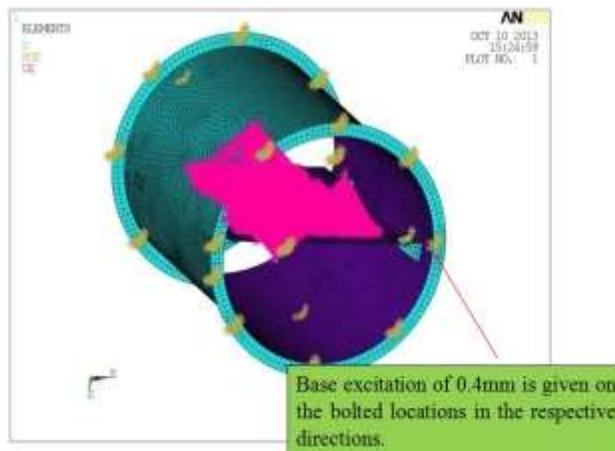
Fig 45 Shows Boundary conditions applied on the mounting structure for RSA analysis
