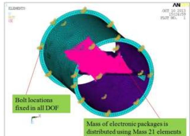
Fig 23 shows boundary conditions applied on the mounting structure for modal analysis
