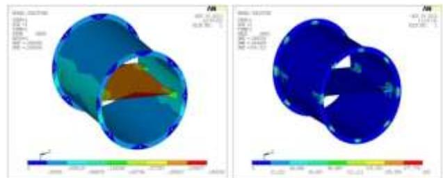
Fig 16 shows deflections & stress plot of mounting structure for pitch condition
