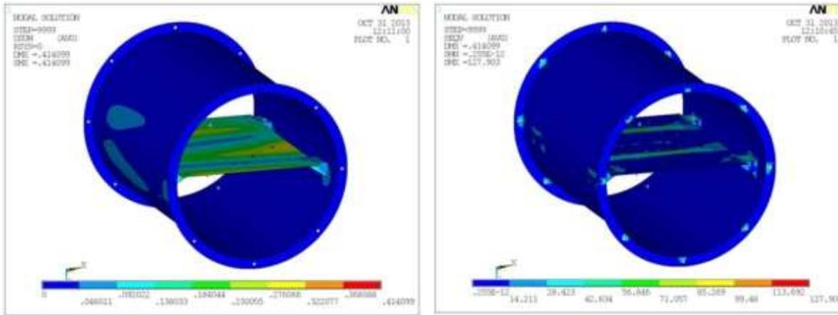
Deflections & Stress plot of mounting structure for Y-Direction
