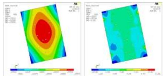
Fig 13 shows deflections & stress plot of mounting plate for yaw condition
