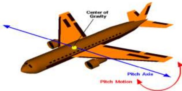
Figure 3 Flight vehicle- Pitch motion
