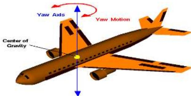
Figure 5 flight vehicle- yaw motion
