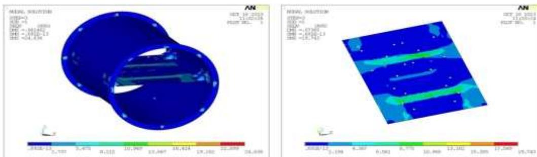
Fig 35 shows 1 sigma stress for PSD analysis in Y-Direction
