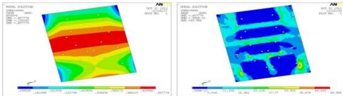
Fig 53 shows Deflections & Stress plot of mounting plate for Z-Direction
