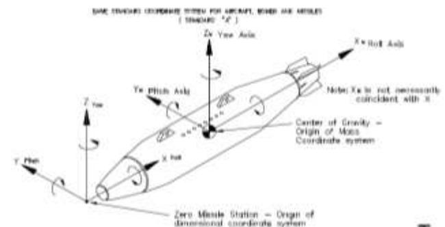
Figure 2 Three modes of motion in a flight vehicle
