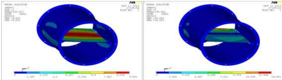
Fig 24 shows the 1<sup>st</sup> and 2<sup>nd</sup> mode shapes for modal analysis
