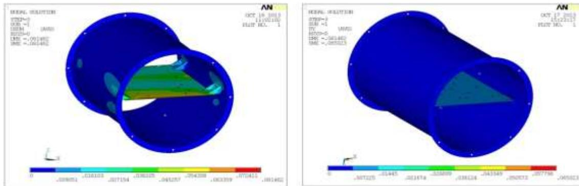
Fig 34 shows 1 sigma displacement for PSD analysis in Y-Direction
