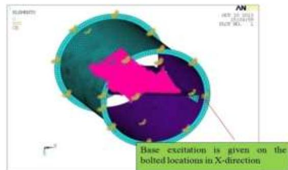
Fig 27 shows Boundary conditions applied on the mounting structure for PSD analysis in X-Direction
