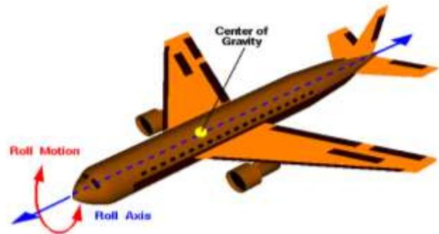
Figure 4 flight vehicle- roll motion
