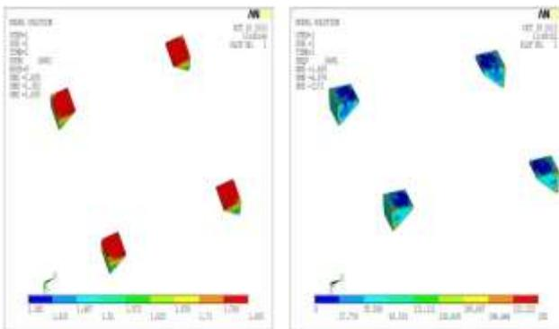
Fig 22 shows deflections & stress plot of lugs for roll condition
