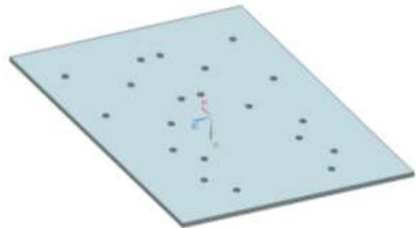
Fig 9 shows the 3d model mounting structure plate.
