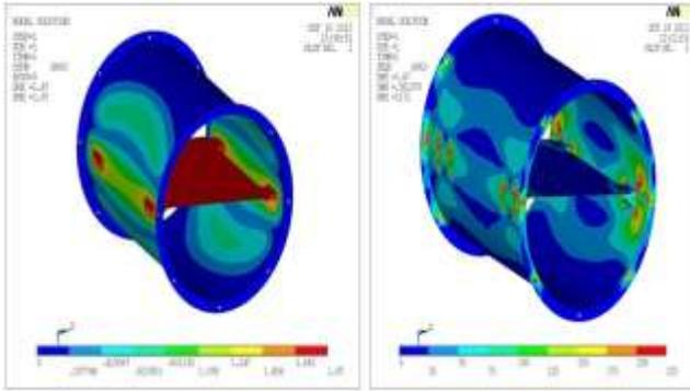
Fig 20 shows deflections & stress plot of mounting structure for roll condition
