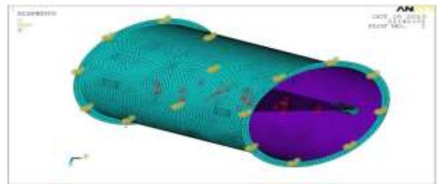
Fig 11 shows boundary conditions applied on the mounting structure for yaw condition
