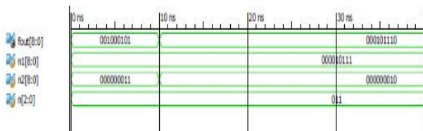
Figure 12: Timing Waveform of RNS based Multiplier Unit
