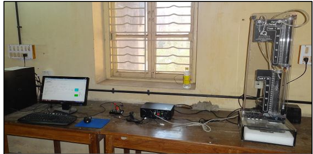
Fig: 2 Real time water tank system
