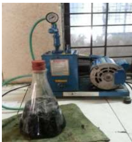
Fig 5: Air Voids determination setup
