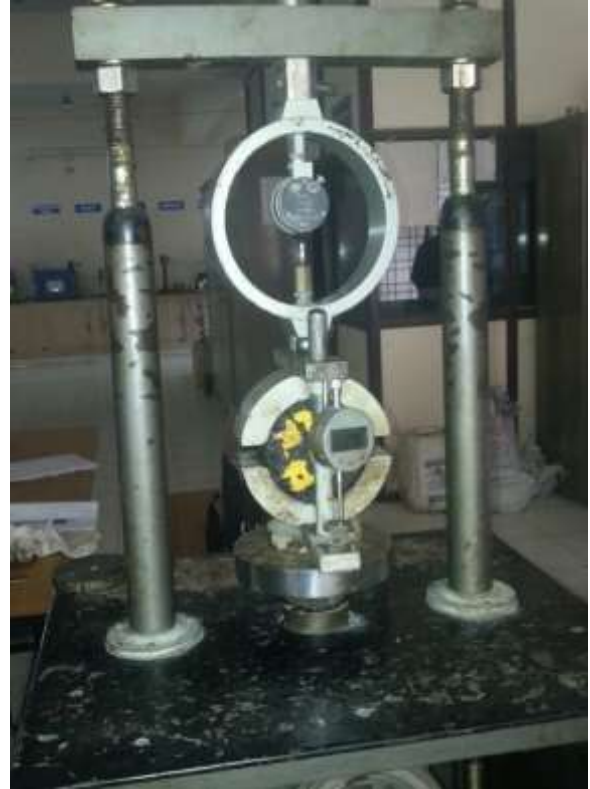
Fig 4: Marshall Stability Test Setup
