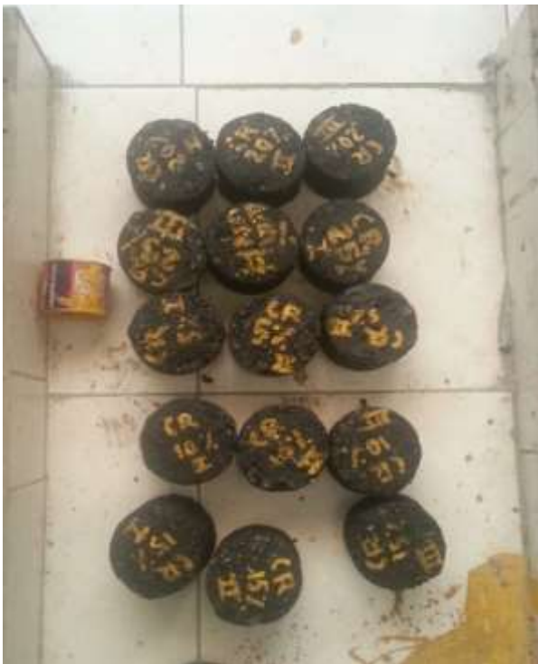
Fig 2: Marshall moulds for OBC determination
