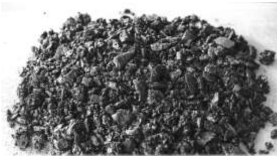
Fig 3: Loose mix(uncompacted) for air voids calculation
