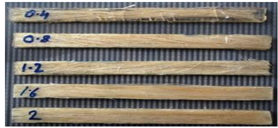
Fig. 6 Sisal fiber composite specimens subjected to tensile testing
