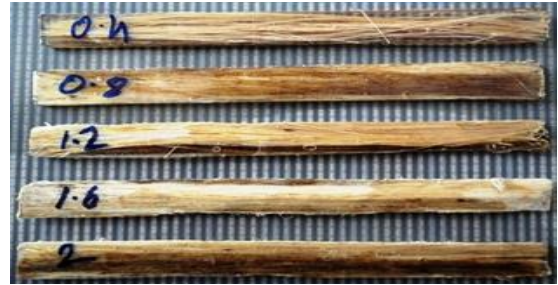
Fig. 7 Hybrid fiber composite specimens subjected to tensile testing
