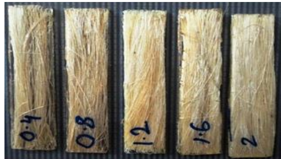
Fig. 8 Sisal fiber composite specimens subjected to flexural testing
