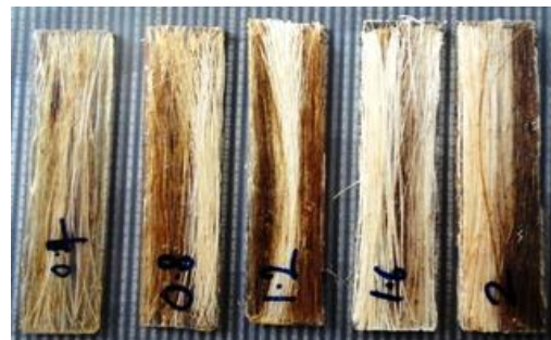
Fig. 9 Hybrid fiber composite specimens subjected to flexural testing
