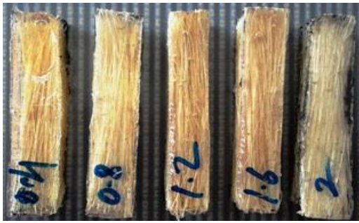
Fig. 10 sisal fiber composite specimens subjected to impact testing
