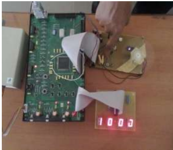
Fig. 6 Experimental setup of FPGA based PID controller for DC motor speed control.
